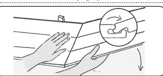
2. Press the next floor plank at an angle of 20° against the first one and lay it down. Continue in the same way along the length of the first row. Cut the last plank in the first row to the correct length and keep the suitable compensation joint. Before installation remove the possible dirt and scrapings. Dirt can cause some tightening and tension in the parquet.
